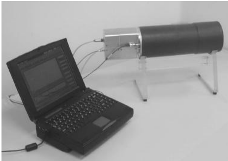
FIGURE 7. Photograph of xenon detector arrangement
